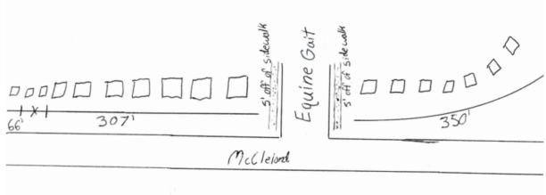
Furnish and install 723' of 6' tall white tongue and groove vinyl privacy style fence. All posts are to be set in concrete. Install fence 5' off of the sidewalks.
